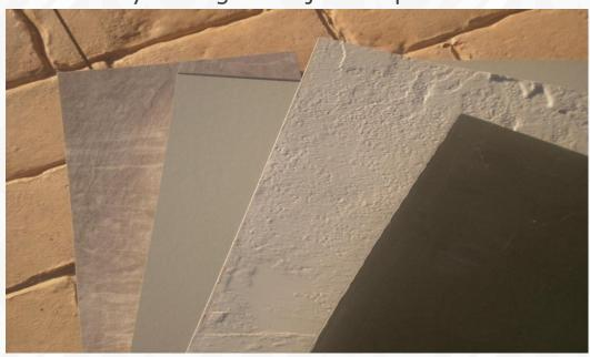
Panel manufacturing occurs in an industrialized process, by using injection molding machines and pressed polyurethane foam by the process or machine cast-against-injection mold.
